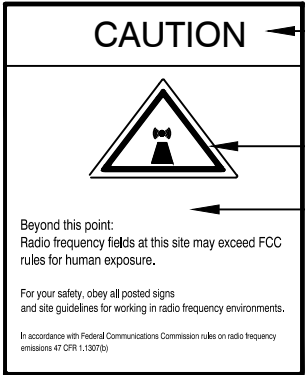
2 RF EXPOSURE CAUTION SIGN
